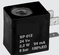
Coil with 2.2 W power consumption 23-SP-012-... page 4.280
