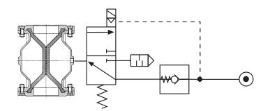
By using a protection circuit a closed air operated pinch valve will stay closed if the compressed air / power supply fails.
