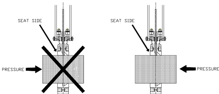
It should be noted that the direction of flow and differential pressure, do not always coincide.
