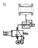
3/2-way solenoid valve (NC) with quick exhaust valve
