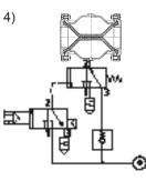
For pressure power shut down: Pinch valve remains in closed position.
