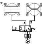
5/2-way solenoid valve for various regulation
