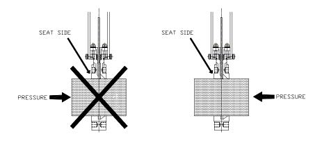
It should be noted that the direction of flow and differential pressure, do not always coincide.
